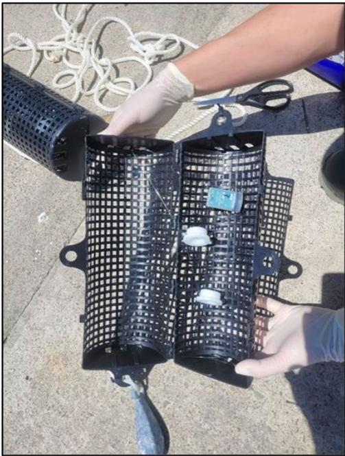
Figure 3 Diffuse Gradients in Thin-film (DGTs) passive samplers (round white samplers) and one temperature logger (Onset® HOBO 64k temperature / light logger, green pendant) contained in cages deployed along mussel frames.
