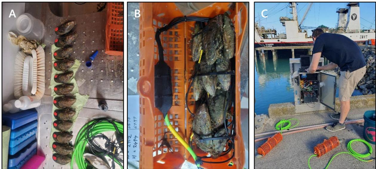
Figure 4 (A) Mussels primed for attachment of Hall sensors. (B) Hall sensors attached to mussels in cage. (C) Shaun Graham (Cawthron) wiring up Hall sensors and deploying them at Layup 3.
