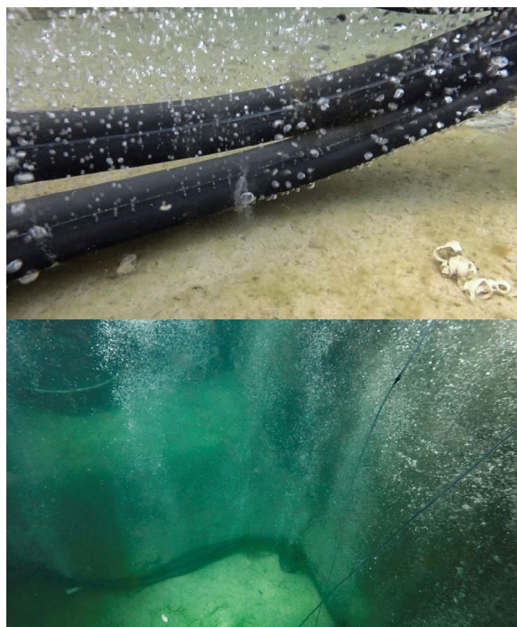
Figure 17. Aeration tests showing bubble production by the Canadian pond aeration tubing (upper) and surface view of the resulting bubble curtain (lower).
