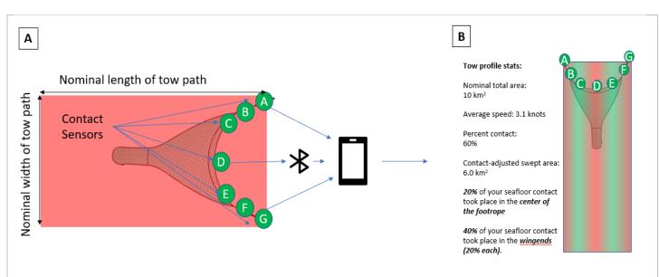
Figure 2 Demonstration of how the sensors are used to develop more high-resolution fishing footprints. Rather than a swept area just using the nominal width of the tow path and the nominal length of the tow path (Panel A), the sensors will inform what portions of the net are making direct contact during a tow (Panel B).
