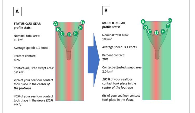
Figure 3 How modifications to status-quo gear (Panel A) can result in improvements in contact (Panel B) with modified gear, using the results of measuring the status quo gear to inform the modifications.
