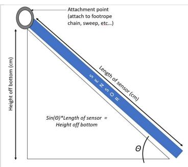
Figure 1 Generic sensor design, and explanation of how the sensor works.
