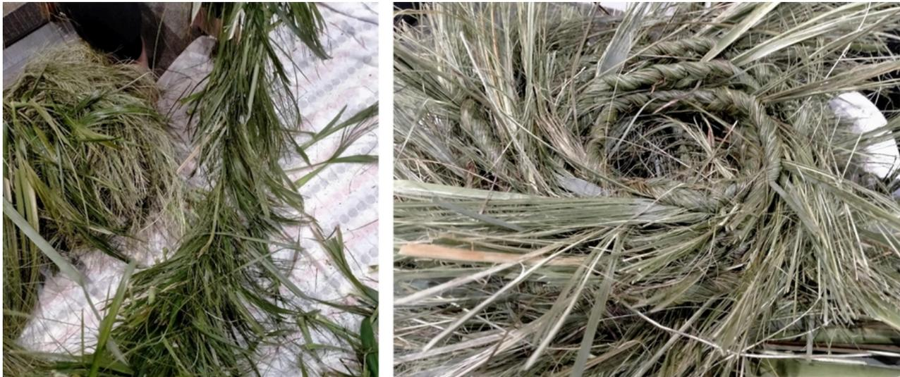
**Fig. 2.** Photographs of natural fibre ropes manufactured by plaiting techniques by iwi project partners, Ngāti Manuhiri (left - harakeke, right - tī kōuka) that were used for assessing fibre resistance to seawater.
