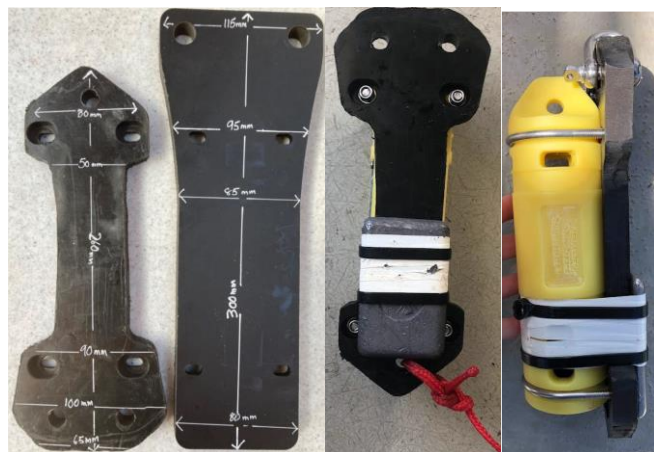
Figure 3 Photo demonstrating the reduced surface area of the plate attached to the sensor to minimize any hydrodynamic lift, as well as added weight
