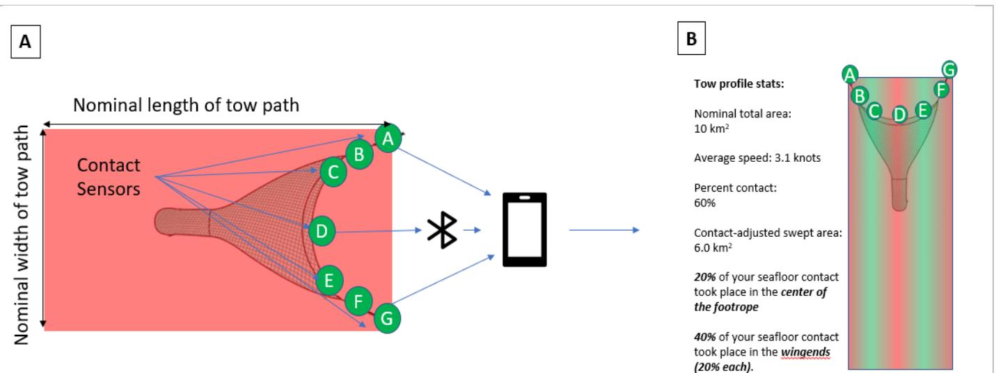
Figure 2 Demonstration of how the sensors are used to develop more high-resolution fishing footprints. Rather than a swept area just using the nominal width of the tow path and the nominal length of the tow path (Panel A), the sensors will inform what portions of the net are making direct contact during a tow (Panel B).
