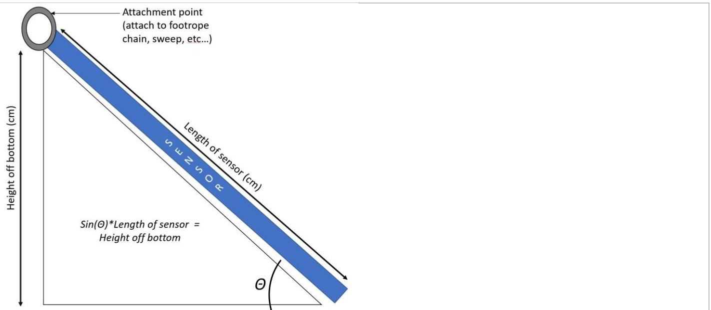
Figure 1 Generic sensor design, and explanation of how the sensor works.
