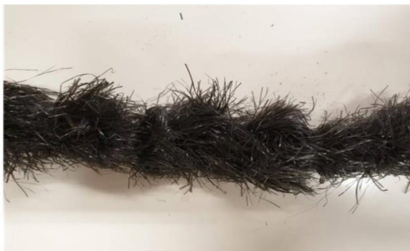
Figure 1. Example of a commercial spat catching rope widely used in the Greenshell™ aquaculture industry which consists of cut strands of polypropylene to simulate filamentous seaweed and hydroids onto which spat normally prefers to settle in the wild. Note the plastic particles lying around the rope that have been shed from the rope with handling.
