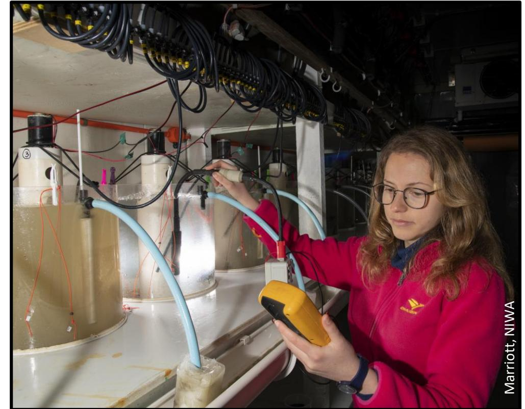
Manual checks (optical turbidity meter)
