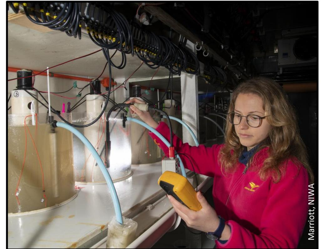
Manual checks (optical turbidity meter)
